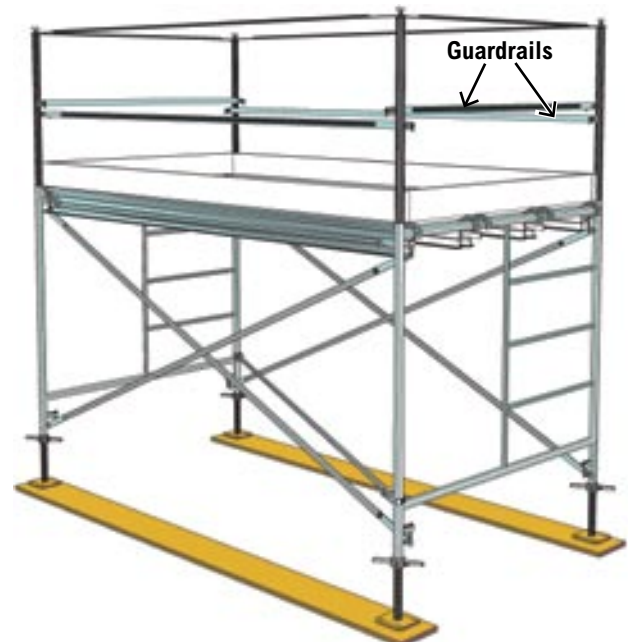
This is an example of a metal guardrail system.
