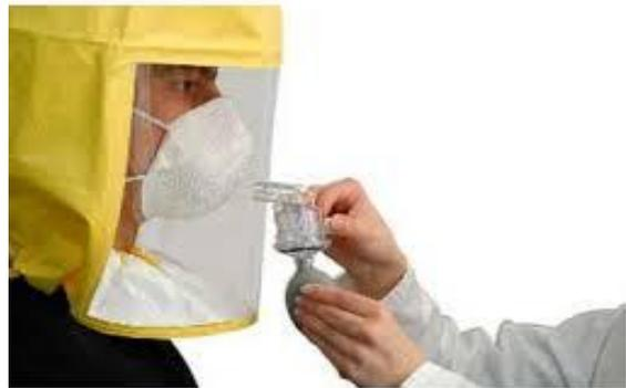
In order to do these measurements, a small sampling tube is positioned to sample the air within the face piece of the respirator and attached to a fit testing instrument able to calculate the percentage of particles leaking into the face piece.
