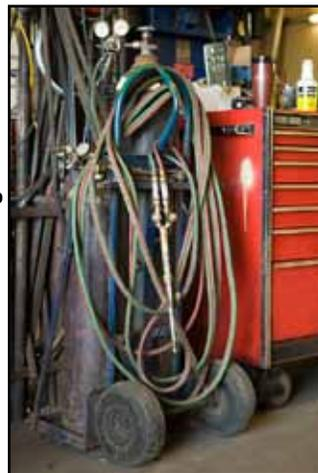
**The hoses on this welder are neatly wrapped around the equipment and stored they remain out of the aisle.**
