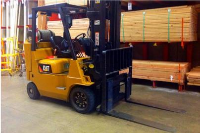
Every powered industrial truck has a placard from the manufacturer indicating the lifting capacity of the vehicle based on its engineered design and attachments. One of the key responsibilities of any operator of such equipment is to know that capacity and ensure they don't exceed it by lifting objects
