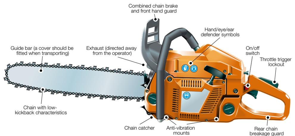
Figure 1 Rear-handled chainsaw
